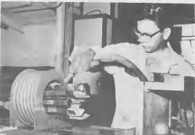
PAVEMENT BREAKERS' bits receive the magnaflex treatment directed by Alexander DeKort, a six-month trainee from HTS in Breda, Holland. Mr. DeKort will spend three months with the Equipment Inspection Group and three months in Process-Engineering.
